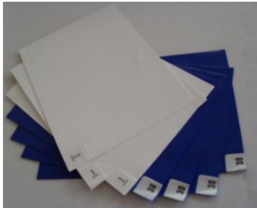
**Stack of sheets of polyethylene, with a specially treated sensitive adhesive on one side, upon which persons entering a clean room or clean zone walk to remove the last trace of contamination on shoe heel and soles, and on wheels. When a sheet becomes loaded with contamination, it is peeled off, exposing a new clean sheet**
